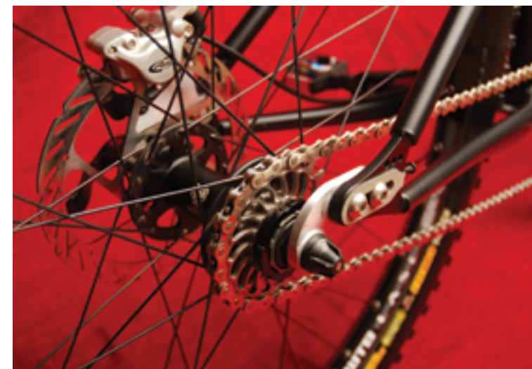
Ground Up Designs recommends using blue Loctite on the sliding dropout bolts.
