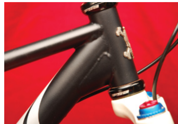
The TIG welded head tube gusset allows for plenty of fork crown clearance.
